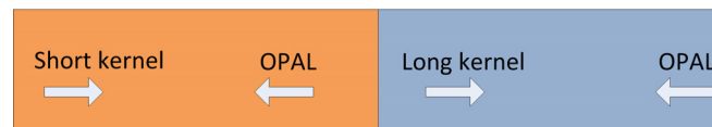
Fig 2. Database processing steps. Sequences in the database are sorted by their length and divided into two partitions. In the both partitions GPU kernels (short and long) process from shorter to longer sequences and OPAL (CPU implementation) processes in the opposite direction.
