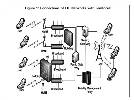
Serving gateway provides routing and forwarding functionality among the macrocell, femtocell and packet data network (Acakpovi *et al.*, 2013). It supports routing of data. Femtocells and macro cells are connected to the mobile core network by serving gateway which behaves like a mediator for signaling control (Lee and Lin, 2010). Mobility management provides the correct serving gateway to the user equipment. Mobility Management Entity (MME) also authenticates the users.
