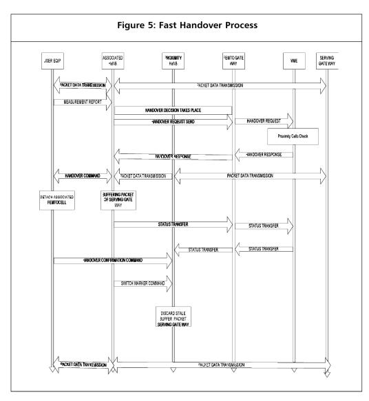
ready to attach itself to target femtocell. Now the source femtocell buffers packets which are received from serving gateway and sends the status transfer message to the target femtocell, followed with switch marker. Switch marker discards the already received packets. Now the handover is confirmed between target femtocell and the user equipment. This is called fast handover process due to switch marker command.
