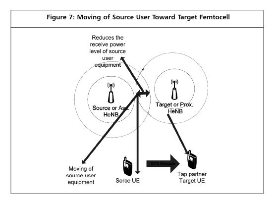
equipment id and source femtocell id (Dampage and Wavegedara, 2013). The direct transfer of handover request to target femtocell saves the Internet delay. Takeover process is performed by target femtocell. This process informs the mobile management entity that target femtocell wants to handover with source user equipment. The following steps show the process of handover (Dampage and Wavegedara, 2013).
