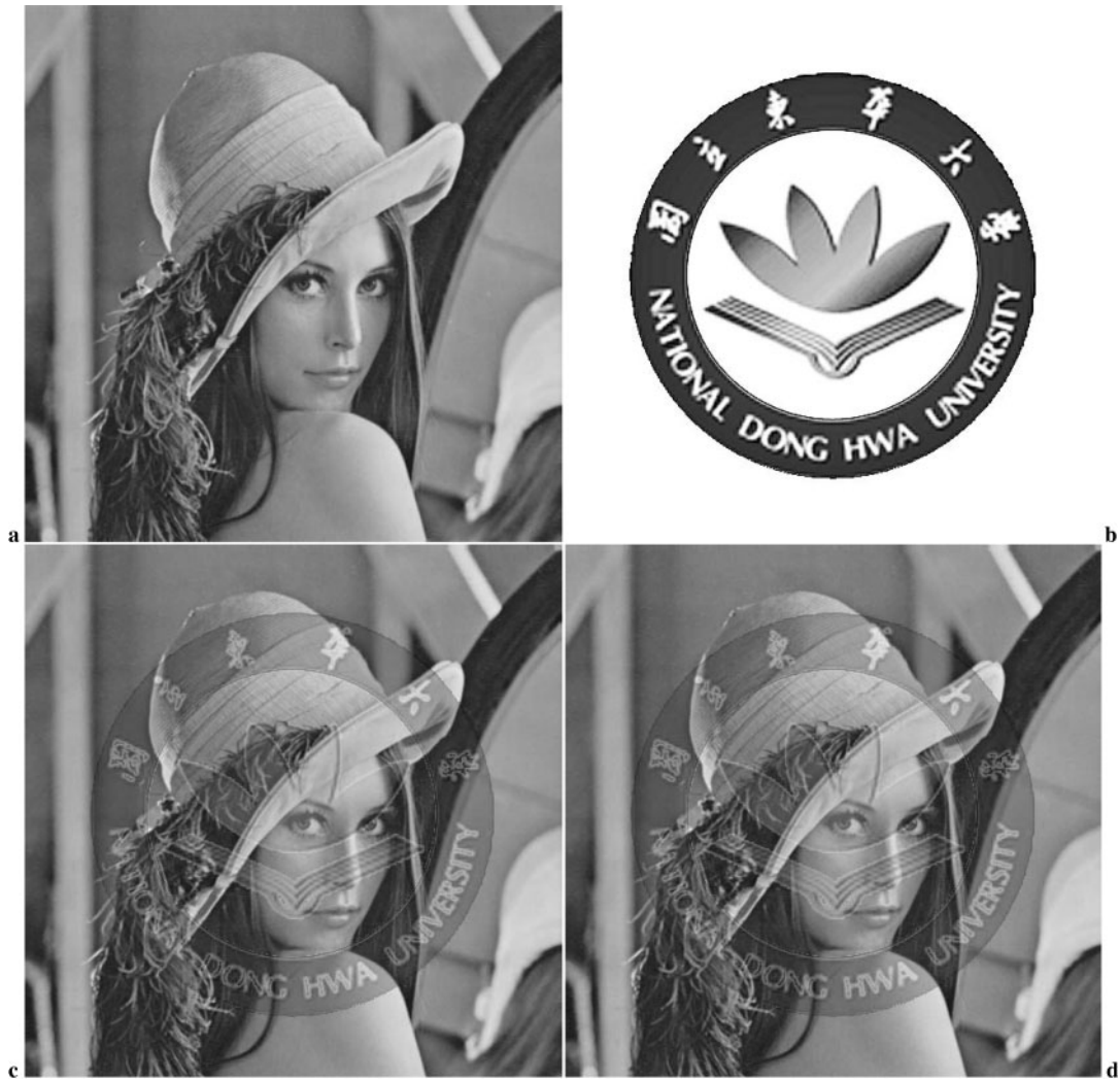
2 a Lena , b watermark pattern, c watermarked Lena (before information hiding) and d final watermarked Lena (after information hiding)
