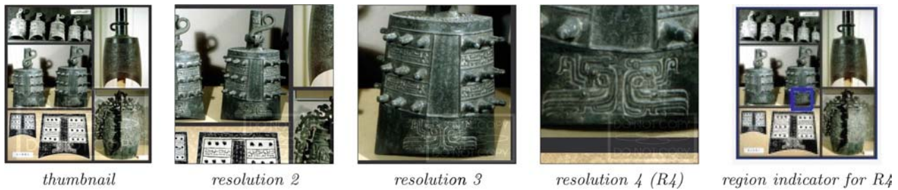
Fig. 7 A user can progressively zoom in the region of interest. The requested region at the requested resolution is dynamically generated from wavelet coefficients. A light visible watermark is added at the lower right corner of the image before transmission
