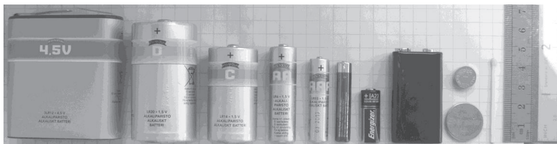
FIGURE 2. Common consumer type battery packages, from left to right: a large 4.5 Volt battery, a D-cell, a C-cell, an AA-cell, an AAA-cell, an AAAA-cell, an A23 battery, a 9 Volt (PP3) battery, and a pair of button cells (CR2032 and LR44). Picture and caption reprinted from [3].
