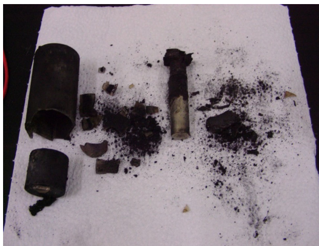
Fig. 5 Battery severely ruptured after thermal runaway
