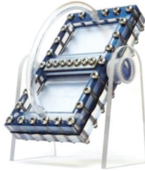
FIGURE 13. The Gravity Induced Flow (GIF) cell, where anode and cathode liquid solutions or suspensions in the tanks flow past the reaction plate or “stack” under the influence of gravity. A small motor (not shown) replaces the pumps that drive the liquids in a conventional flow battery, adjusting the tilt of the GIF cell and controlling the flow rate.
