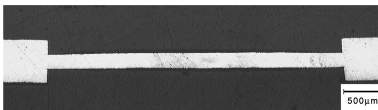
Figure 7. DTE-bonded sample showing minimal fin warpage.
