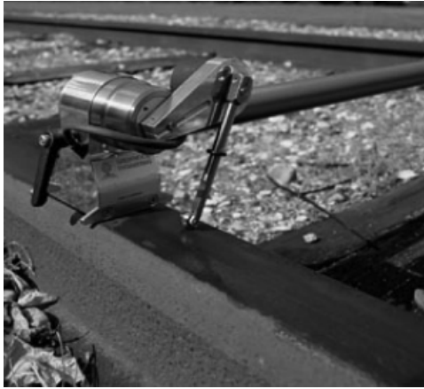
Fig. 1. Rail Profile Measurement [MINIPROF, Greenwood, Denmark].
