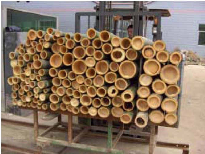
Fig.1. Typical batch of row bamboos collected for producing GluBam
