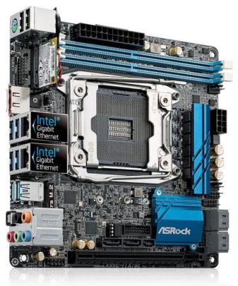
Asrock's X99 MiniITX board simply does away with two memory channels to save space.
