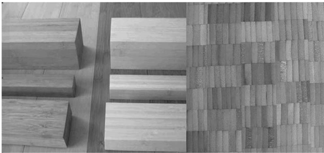
Fig. 5. (Left): Laminated bamboo lumber from manufacturer in China, shipped to United States for many building finishing products (Image courtesy of 4windsbamboo.com); (right): Close-up of bamboo lumber section made up of many strips laminated together (Rittironk and Elnieiri 2007; reprinted with permission from CRC Press/Taylor and Francis Group)
