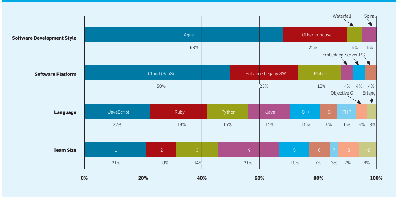
Figure 4. Survey results of software experience for former Berkeley students now in industry. (The waterfall software development process is characterized by much of the design being done in advance of coding, completing each phase before going on to the next one. The spiral model combines features of a prototyping model with the waterfall model and is intended for large projects.)
