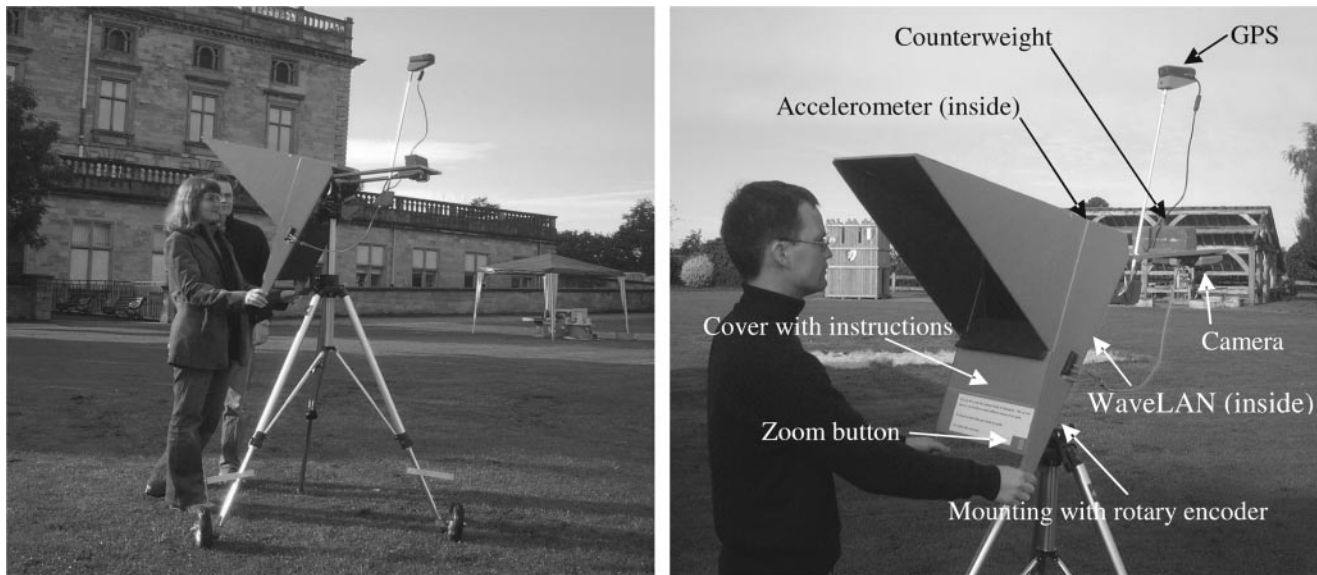
Figure 2. Augurscope 1: overview and detail of top unit.
