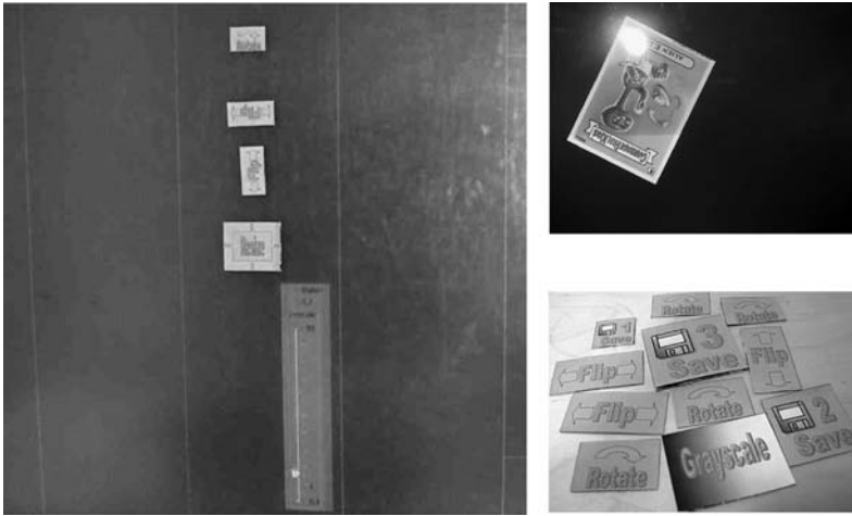
Figure 13. SiteView, a spatial UI for end-user control of home automation systems. Left: A physical light-bulb icon on the floor plan, with projected feedback above. Right: The six physical icons.
