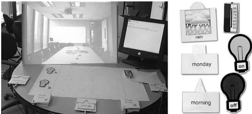
Figure 13. SiteView, a spatial UI for end-user control of home automation systems. Left: A physical light-bulb icon on the floor plan, with projected feedback above. Right: The six physical icons.
