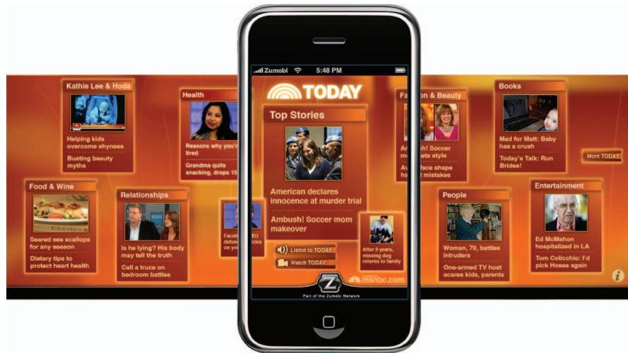
Figure 2. Recent ZUI: Zumobi’s ZoomCanvas zooms in from the entire canvas on start-up. Dragging left/right pans, and tapping on a region zooms in for interaction with the detailed content (Zumobi 2010).
