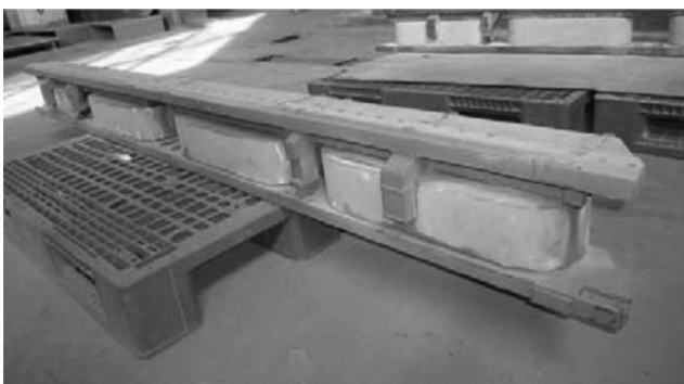
Fig. 7 Photograph of the prototype for the hybrid suspension electromagnet
