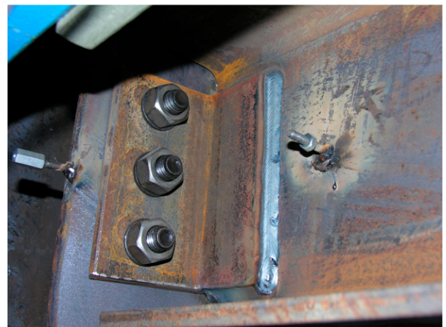
Fig. 5. Shear connection: (a) as fabricated; (b) at end of test
