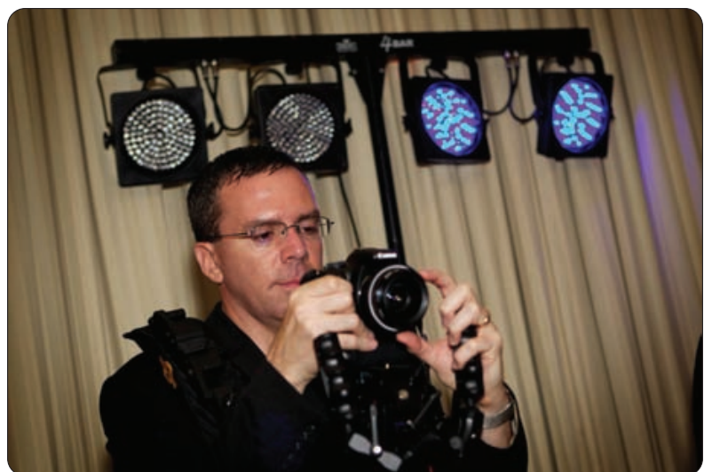
The DVTEC MultiRigPro with handgrips positions up close to the camera. Note how I use the right grip to hold on to the rig and the camera at the same time, leaving my left hand free to focus.
