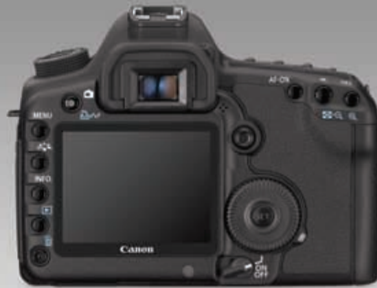
Canon's new 60D (left) is the first Canon DSLR to feature a camcorder-style articulating LCD screen; previous Canon models such as the 5D Mark II (right) use a fixed LCD, which limits where shooters can position themselves to monitor their shots.
