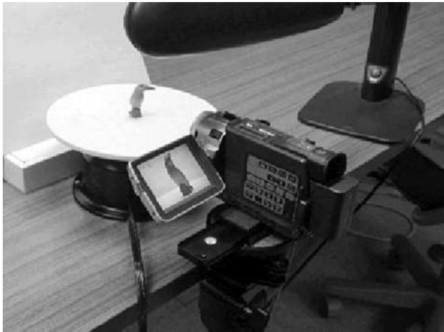
Figure 9. Equipment for capturing turnoramas.
