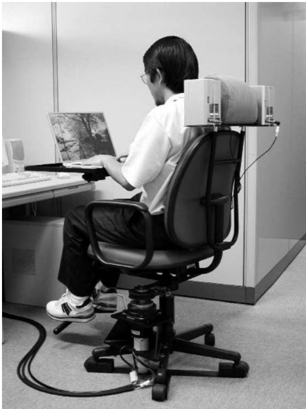
Figure 3. Internet Chair integrated with VR 4 U 2 C : The swivel chair is a rotary motion platform. The panorama displayed by the laptop computer (with wireless internet connectivity) is proprioceptively anchored, panning opposite to the chair rotation driven by the servomotor and the soundscape displayed through “nearphones,” loudspeakers straddling the headrest for binaural display without crosstalk. (Developed by the first author and Uresh Duminduwardena with the collaboration of Yamagata University and Mechtec.)
