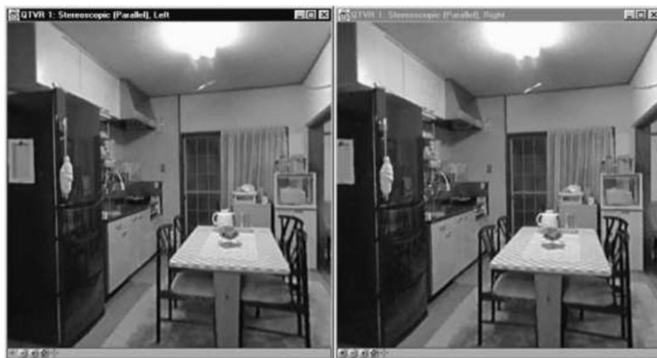
Figure 7. Example of left/right stereo images. Note binocular parallax viewpoint displacement, causing offset of objects like the paper on the left edge.
