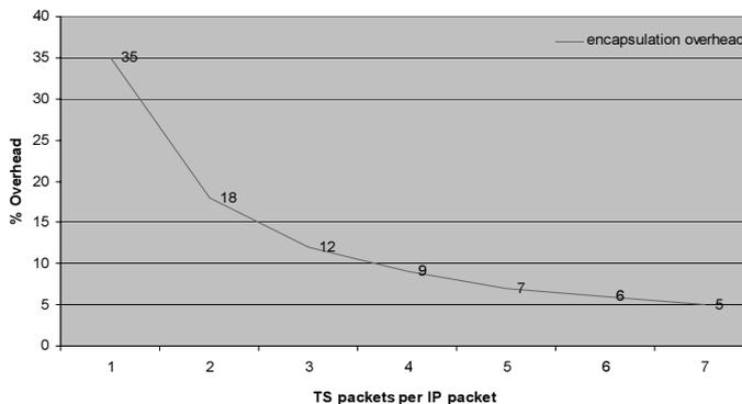
Figure 0 – Transmission overhead vs. packing ratio
