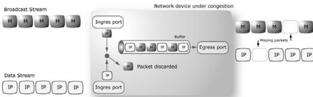
Figure 1 – High Utilization (no QoS)
