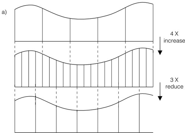
**Fig 3.3.1 a)** A fractional ratio converter can be thought of as two integer ratio converters in series.
