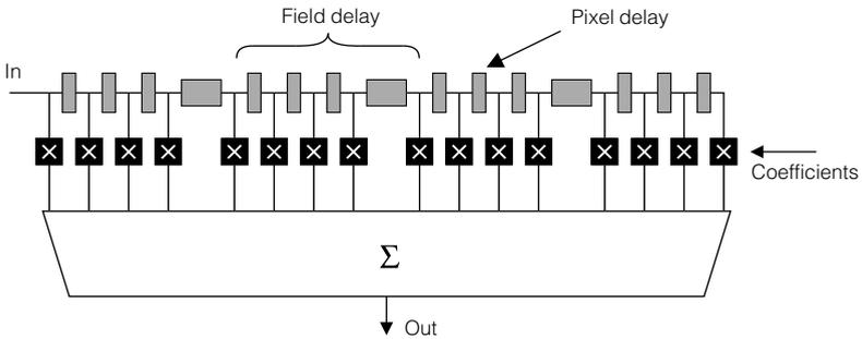
**Fig 3.5.4 a)** A four line by four field two dimensional filter. The location of input samples in the vertical/temporal space is shown in b) overleaf.
