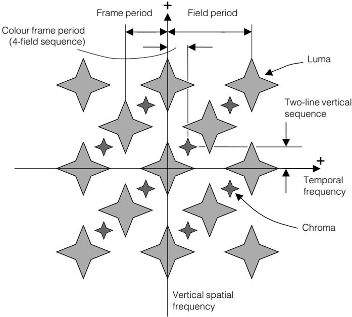
**Fig 2.8.2** Vertical/temporal spectrum of NTSC shows the spectral interleave of luminance and chroma.
