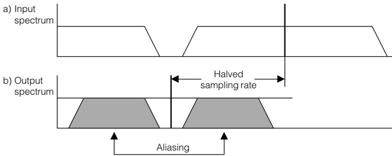
**Fig 3.1.3 a)** Is the spectrum of a sampled system. Reducing the sampling rate alone causes aliasing b) as the sidebands are unchanged in width.
