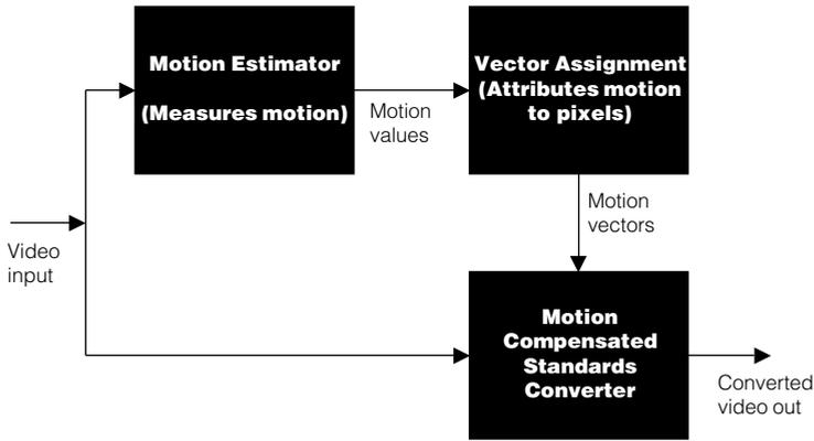
**Fig 3.7.6** The essential stages of a motion compensated standards converter.
