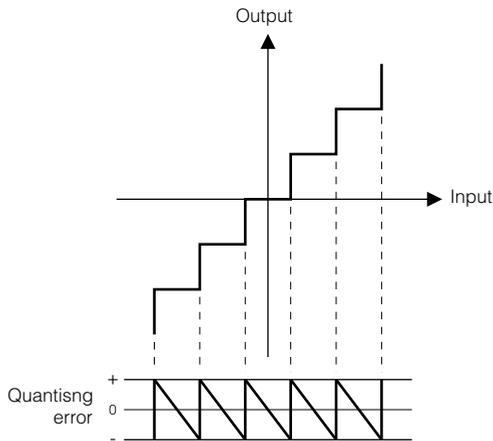
**Fig 2.6.1** Transfer function of an ideal ADC followed by an ideal DAC is a staircase as shown here. Quantizing error is a saw tooth-like function of input voltage.
