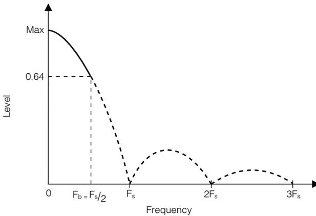
**Fig 2.2.1** Aperture effect. An aperture ratio of 100% causes the frequency response to fall to zero at the sampling rate. Reducing the aperture ratio reduces the loss at the band edge.
