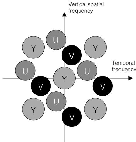
**Fig 2.9.2** A vertical temporal filter with the response shown has better performance on PAL signals and does not need to be adaptive.
