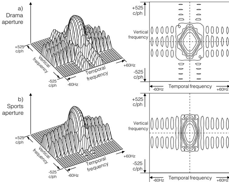
**Fig 3.6.2** The responses of the filter in the ACE converter.
