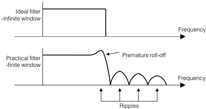
**Fig 2.7.2** The effect of a finite window is to impair the ideal frequency response as shown here.
