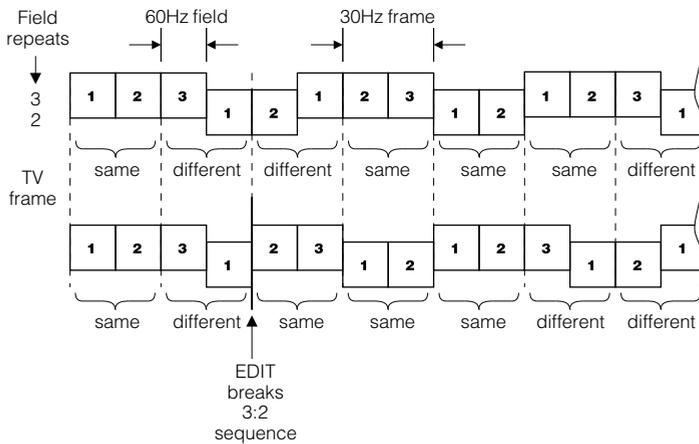
**Fig 4.3.2** In 3:2 pulldown video, there are two types of frame. One type contains two fields from the same film frame. The other contains fields from different frames. A video edit can break the 3:2 sequence and produce a tape with only a single field representing a film frame.
