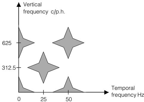
**Fig 3.5.1** The vertical/temporal spectrum of luminance in an interlaced system has a quincunx pattern.
