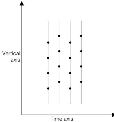
**Fig 3.5.4 b)** The location of input samples in the vertical/temporal space.
