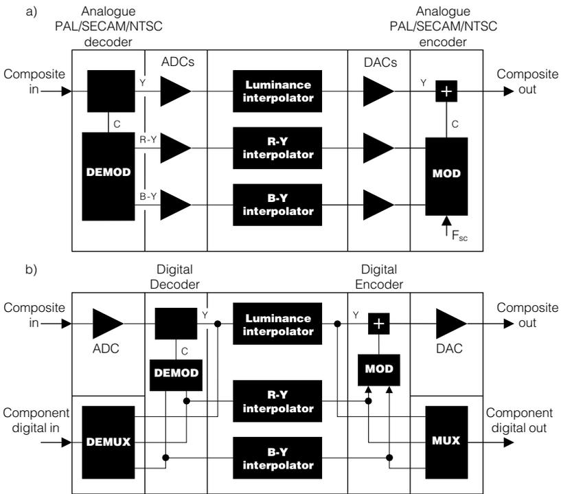
**Fig 1.3.1** Block diagram of digital standards converters. Conversion can only take place on component signals.
