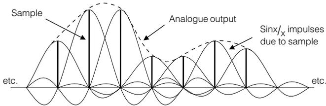
**Fig 3.1.2** In a reconstruction filter, the impulse response is such that it passes through zero at the sites of adjacent samples. Thus the output waveform joins up the tops of the samples as required.
