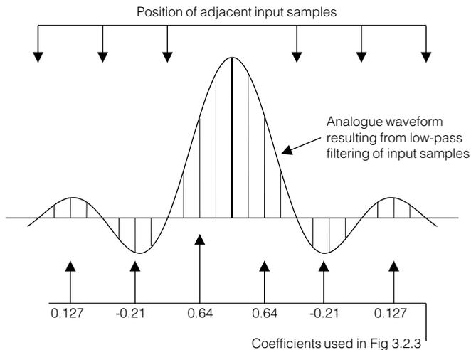
**Fig 3.2.2** The impulse response of the reconstruction filter can be re-sampled at a higher sampling rate to obtain coefficients between existing samples.
