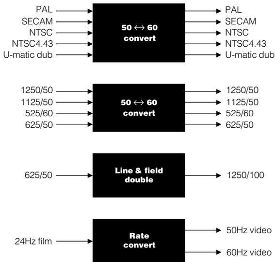
**Fig 1.2.1 a)** Standards converter applications include the classical 525/625 converter
