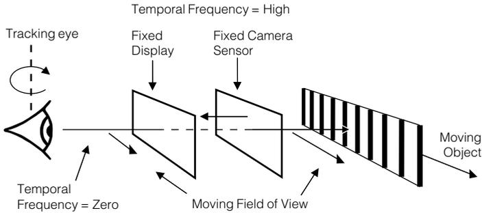
**Fig 3.7.3** An object moves past a camera, and is tracked on a monitor by the eye. The high temporal frequencies cause aliasing in the TV signal, but these are not perceived by the tracking eye as this reduces the temporal frequency to zero. Compare with Fig 3.7.2.
