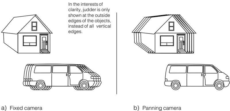
**Fig 3.7.1a)** Conventional four field converter with moving object produces multiple images.
