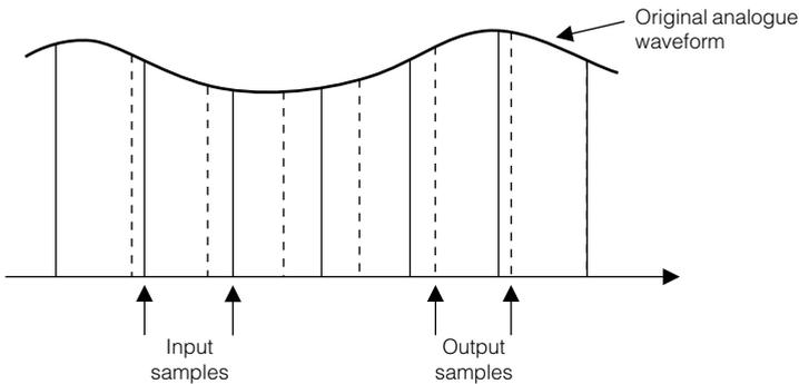
**Fig 3.1.1** Sampling rate conversion consists of expressing the original waveform with samples in different places.
