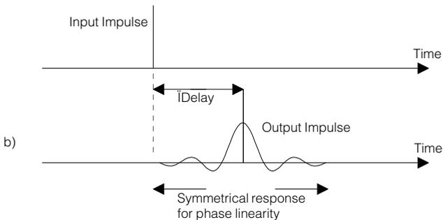
In practice the impulse response is truncated from infinity to some practical time span or window and the filter is arranged to have a fixed delay of half that window so that the correct symmetrical impulse response can be obtained without
