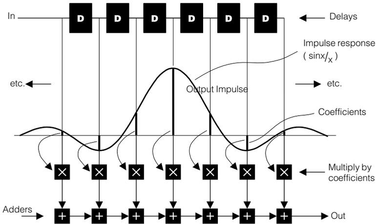
**Fig 2.7.3** An example of a digital low-pass filter. The windowed impulse response is sampled to obtain the coefficients. As the input sample shifts across the register it is multiplied by each coefficient in turn to produce the output impulse.
