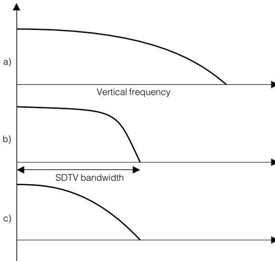
**Fig 2.2.2** Oversampling can be used to reduce the aperture effect in cameras.
