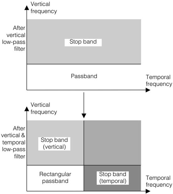
**Fig 3.5.3** If two one-dimensional filters are used, the result can only be a rectangular passband which is of no use in an interlaced system.
