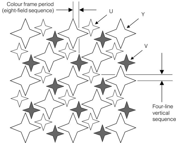
**Fig 2.8.4** The vertical/temporal spectrum of PAL is more complex than that of NTSC because of V-switch.
