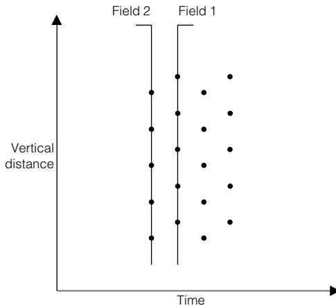
**Fig 2.3.1 a)** In an interlaced system, fields contain half of the lines in a frame as shown in this vertical/temporal diagram.
