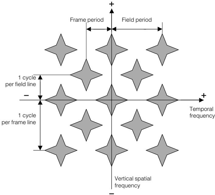
**Fig 2.3.1 b)** The two dimensional spectrum of an interlaced system.
