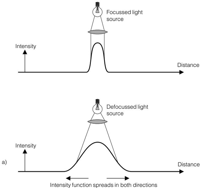
**Fig 2.7.1 a)** When a light beam is defocused, it spreads in all directions. In a scanned system, reproducing the effect requires an output to begin before the input.
