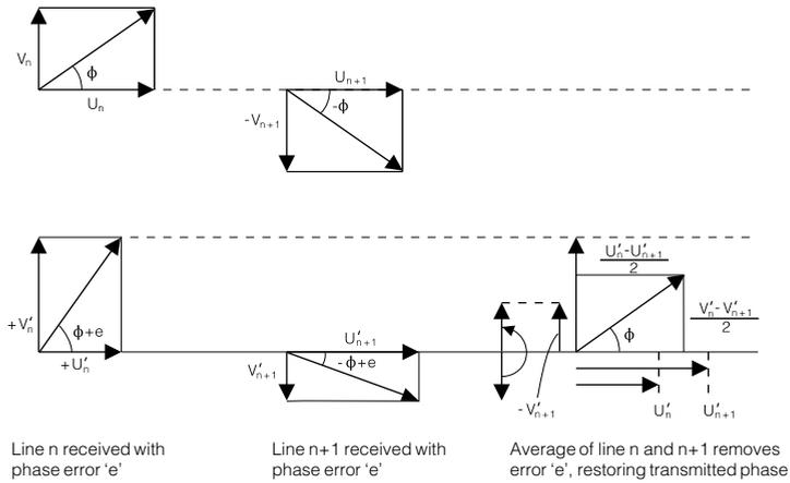
**Fig 2.8.3** In PAL the V signal is inverted on alternate lines. On reception, this turns a static phase error into an alternating amplitude error in U and V which can be averaged out.
