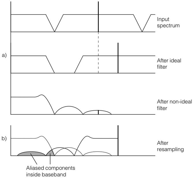
**Fig 3.5.5 a)** With an ideal filter, the images of the input spectrum are rejected and the resampling process produces a clean set of images at the new sampling rate.
