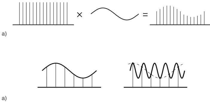
**Fig 2.1.2** Sampling is a modulation process.
