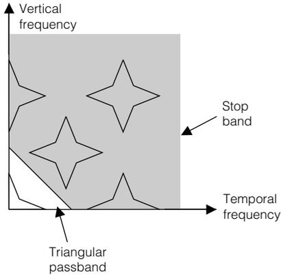
**Fig 3.5.2** In order to return to the baseband in an interlaced system a two-dimensional filter with a triangular response is required.
