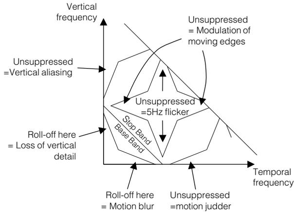
**Fig 3.5.6** Potential problems due to non-ideal filtering are catalogued here.
