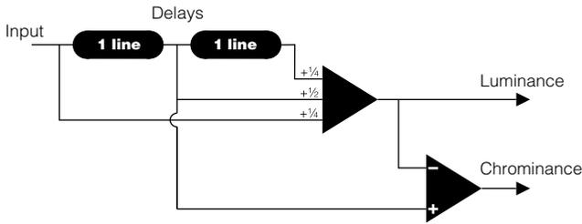
**Fig 2.9.1** A simple line comb filter for Y/C separation needs considerable modification for practical use. See text for details.
