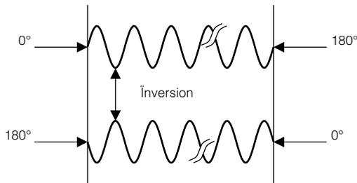
**Fig 2.8.1** The half cycle offset of NTSC subcarrier means that it is inverted on alternate lines. This helps to reduce visibility on monochrome sets.
