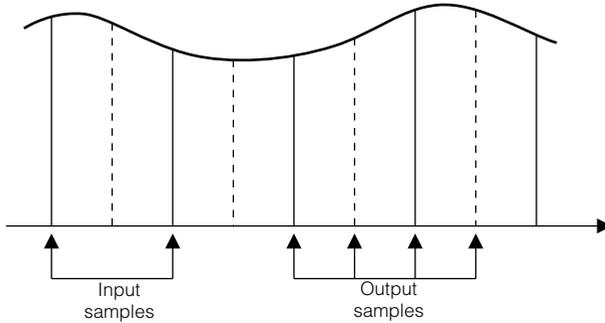
**Fig 3.2.1** In line doubling, half of the output samples are identical to the input samples and only the intermediate values need to be computed.
