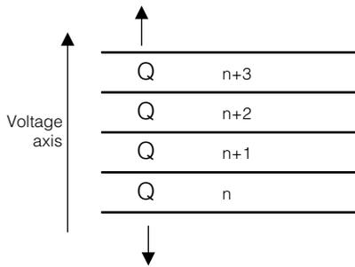
**Fig 2.5.1** Quantizing divides the voltage range up into equal intervals  $Q$ . The quantized value is the number of the interval in which the input voltage falls.
