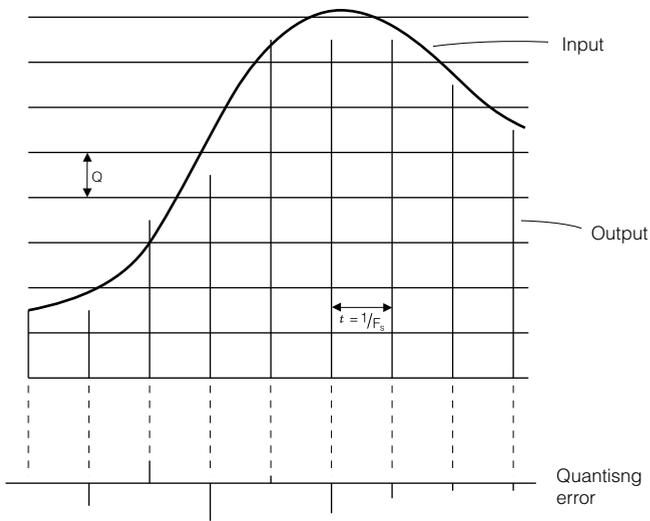
**Fig 2.6.2** Quantizing error is the difference between input and output waveforms as shown here.
