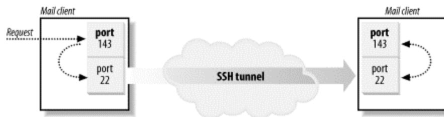
Figure 3-1. IMAP over SSH tunnel
