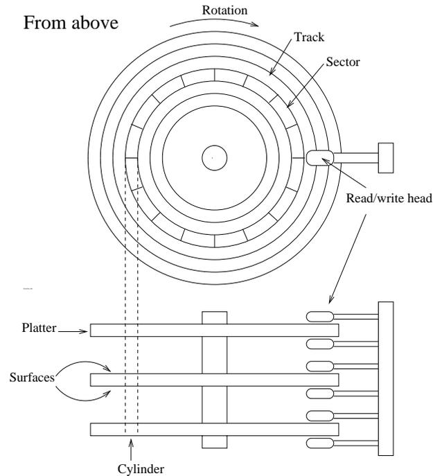
Figure 4.1: A schematic picture of a hard disk.
